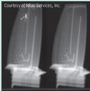
Figure 2.3.3 Neutron radiograph of air-cooled turbine blades
