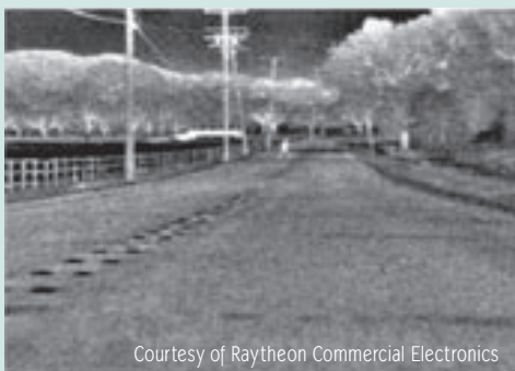
Figure 2.1.2 Pyroelectric Imaging. Lighter colors correspond to warmer temperatures.
