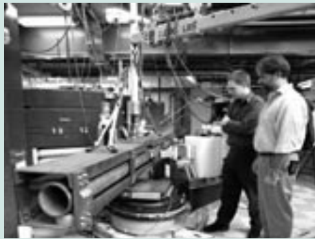
Neutrons can map stresses in a bent water main to validate computer models.
